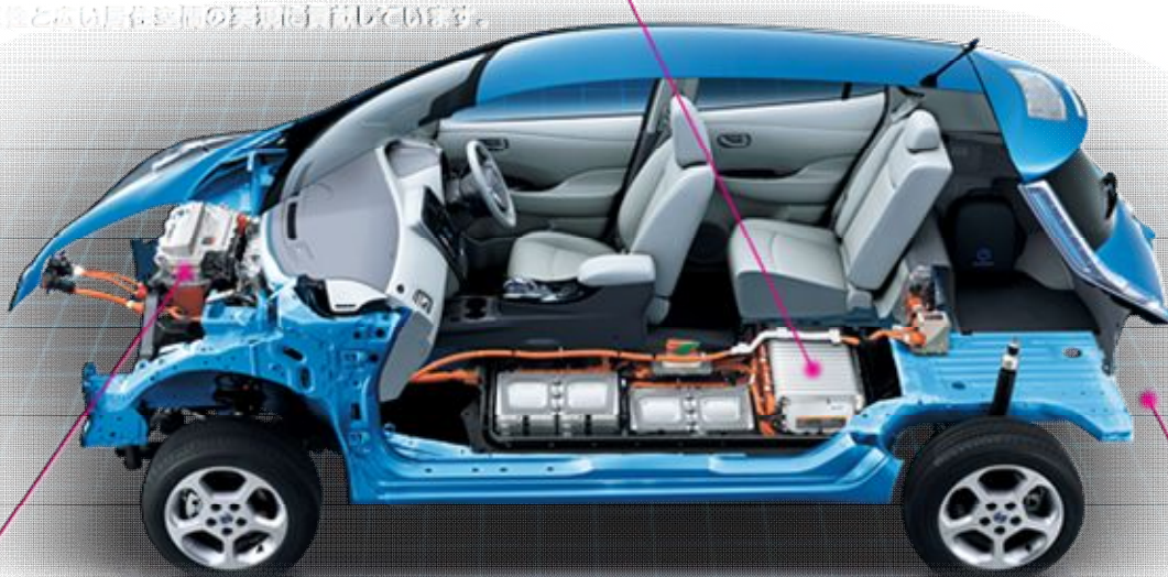
Electric Motor & Inverter
